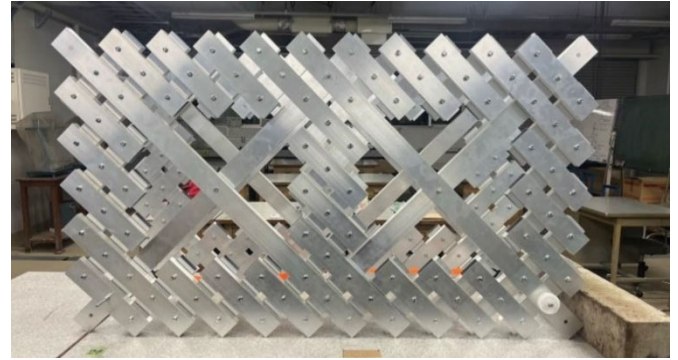
Photo 1. Basic panel of prototype foldable panel bridge
